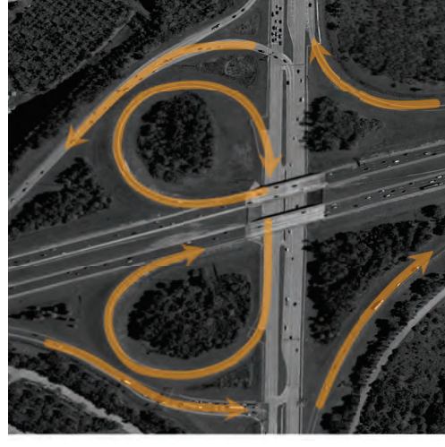
TWO LOOP PARTIAL CLOVERLEAF WITH ACCESS TO AND FROM BOTH SIDES OF SR 836
